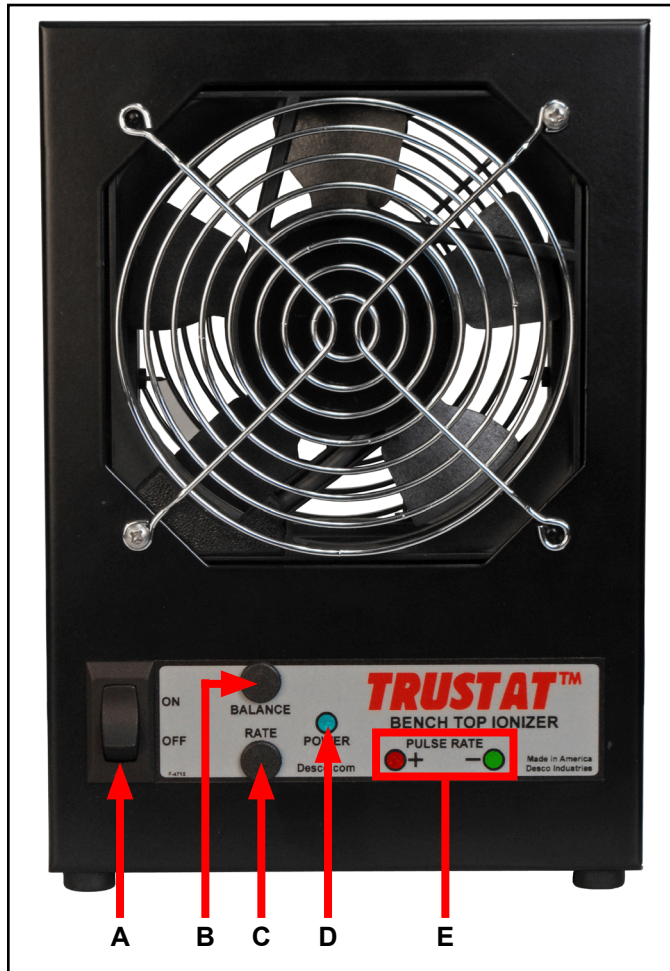
Figure 2. Trustat Bench Top Ionizer features and components
